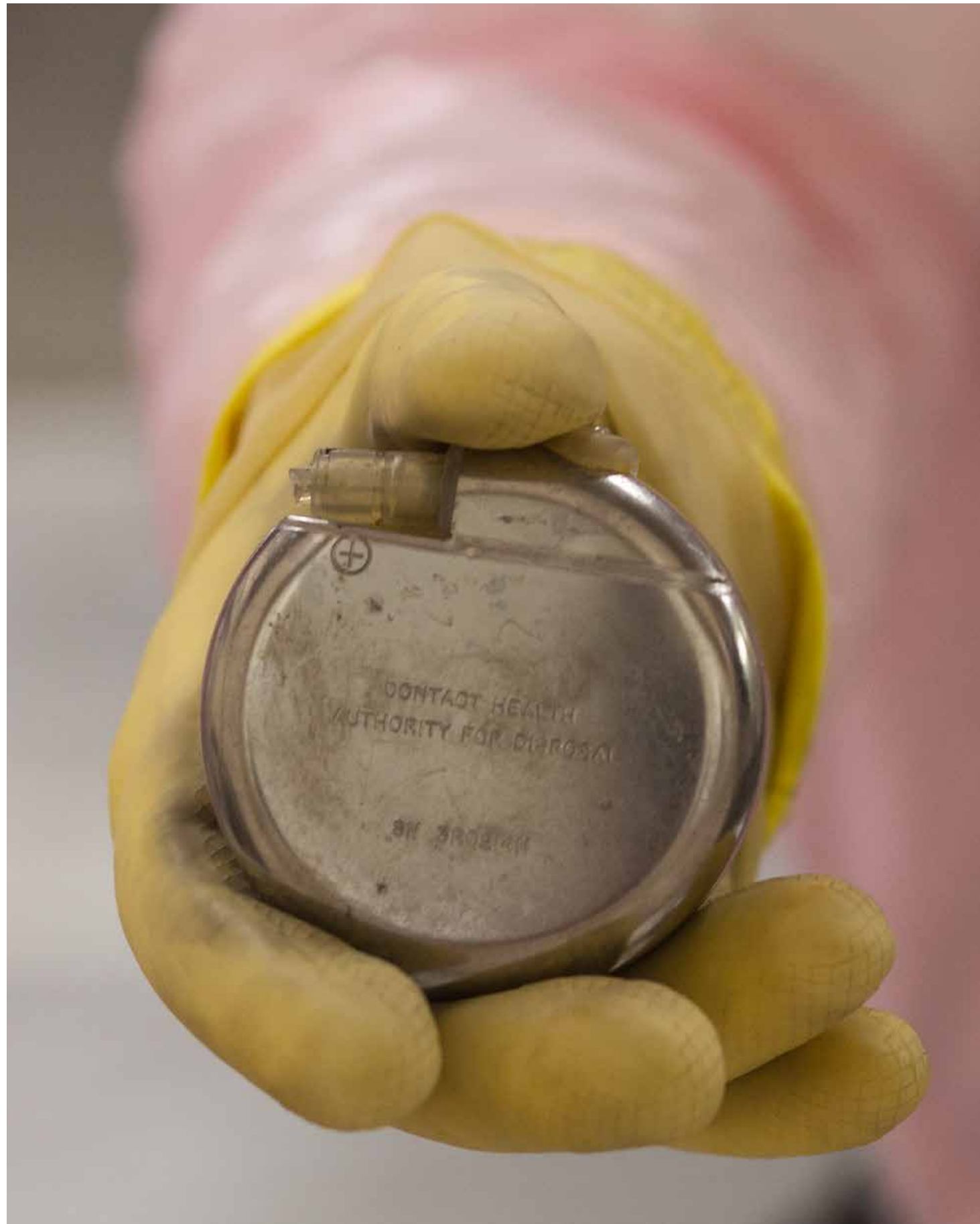
Photograph by Bonsai Publicatiebureau, commissioned by Belgoprocess to document the processing of an explanted plutonium 238 cardiac pacemaker on 11.12.2017
